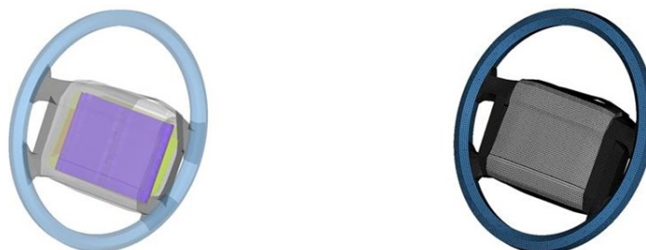
Figure 1: Geometry and mesh model for a steering wheel with closed airbag model.
