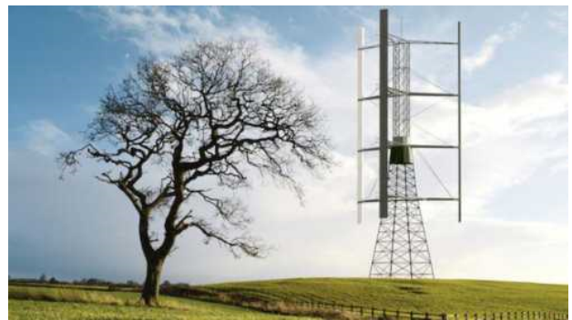
Figure 1: Large scale vertical axis wind turbine (VAWT) (courtesy of Agile Wind Power, Switzerland).
