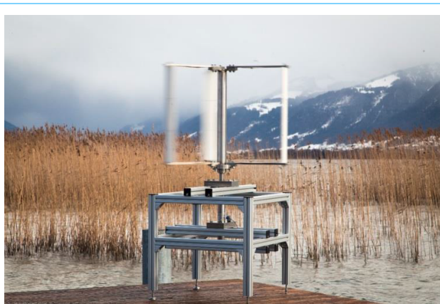
Figure 3: The small VAWT used for the validation studies.
