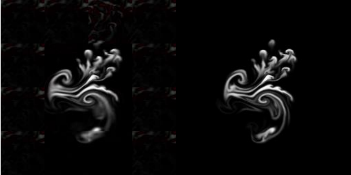
Figure 2: Smoke flow approximated by deep learning (left) vs. accurate MANTAFLOW calculation (right).
